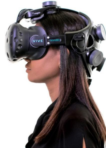
In its current iteration Neurable's EEG headset is an array of seven electrodes that attaches to a HTV Vive headset. (Image source: Neurable)
